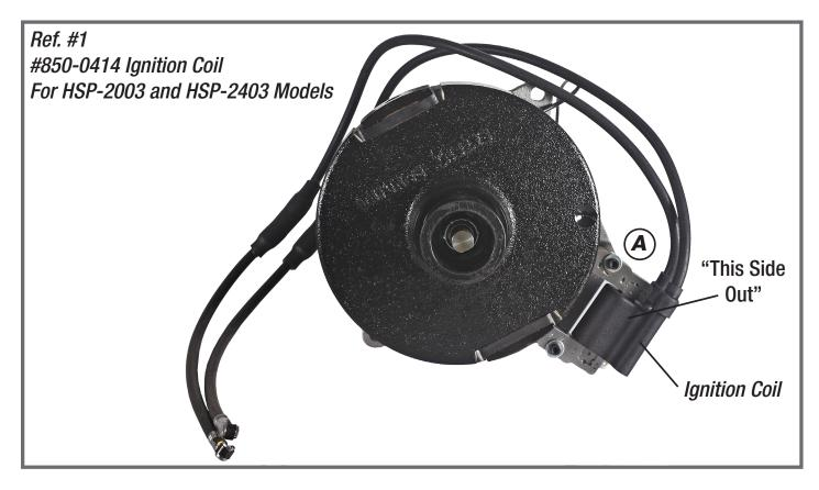
When ignition coil (A) is mounted correctly you can read "this side out." Coil to magnet gap = .010 inch.
